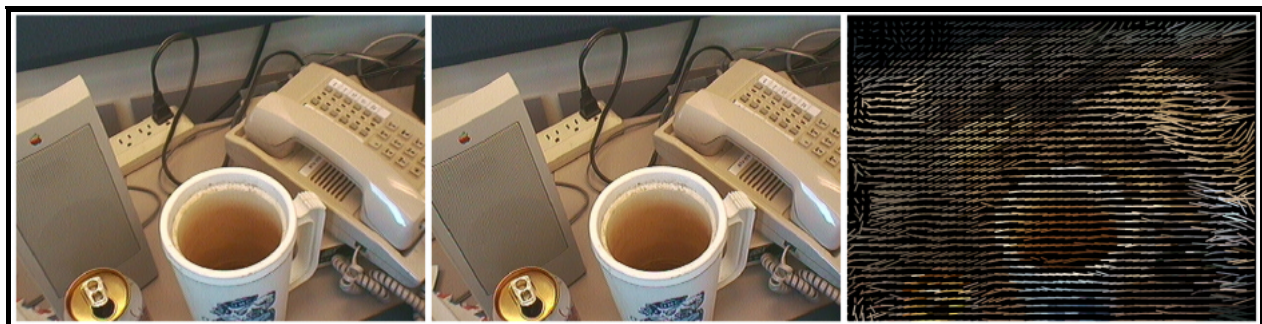
Figure 5. Two frames and the optical flow field that maps pixels from one frame to another.
