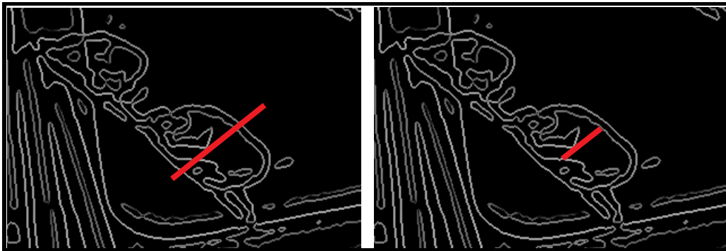
Figure 1. As shown at the left, previous methods have drawn brush strokes without regard to edges. The same brush stroke clipped to edges in the image is shown on the right.
