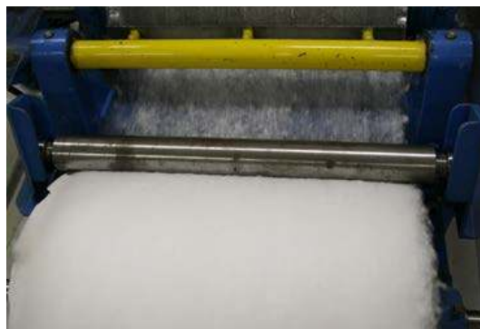
Figure 4. Outlet of the carding machine.
