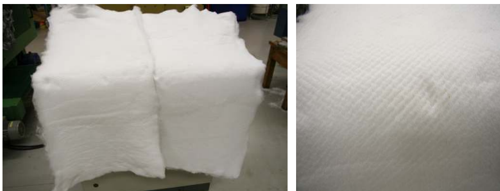
Figure 6. Carded and needled Lyocell mats.
