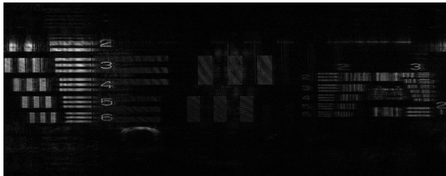
Figure 7. A reconstruction from a synthetic aperture digital hologram of a USAF resolution chart. The aperture has been increased horizontally, giving rise to the horizontally stretched image and higher resolution in that direction.
