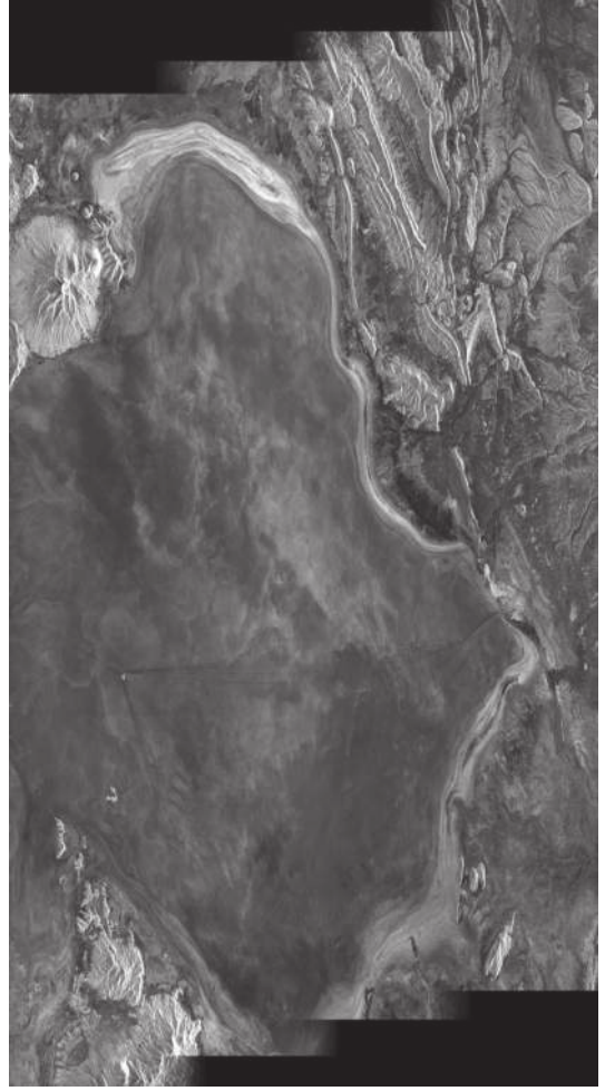
Fig. 9. TOPS image acquired by TerraSAR-X over the Uyuni salt lake, Bolivia. The range is horizontal, and the azimuth is vertical, with near range on the right side. The image dimensions are 120.7 km \times 68.1 km (azimuth \times slant range).
