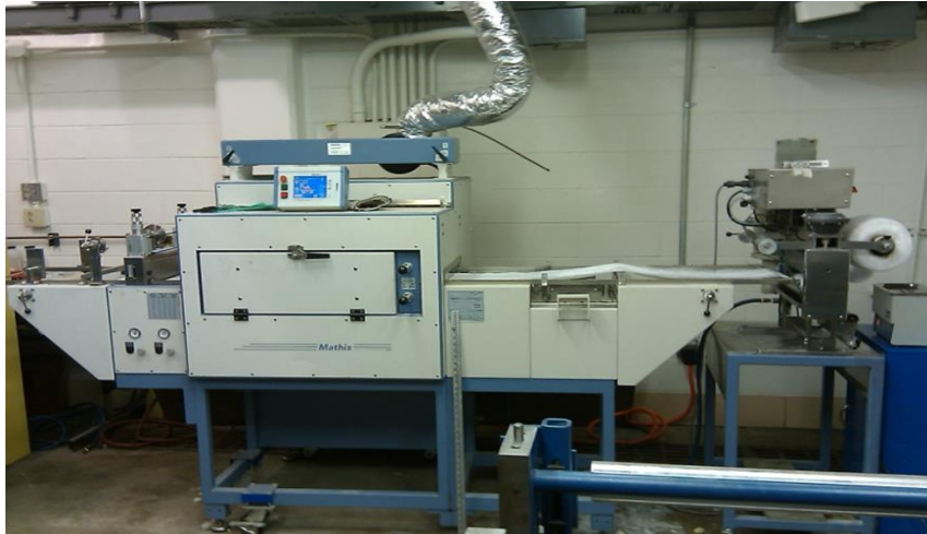
Figure 33. Mathis Coater/Padder/Dryer System
