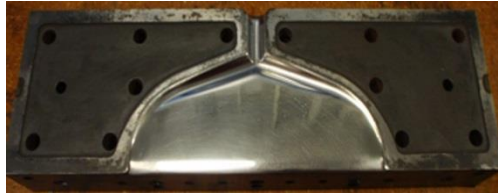
Figure 24. UTNRL 15.4 cm (6 in) melt blowing line coathanger.
