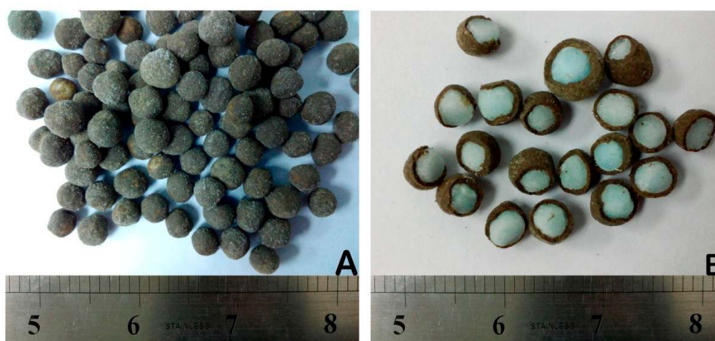
Figure 14. Double coated granules (A) and cross sections (B) of double coated urea (DCU).
