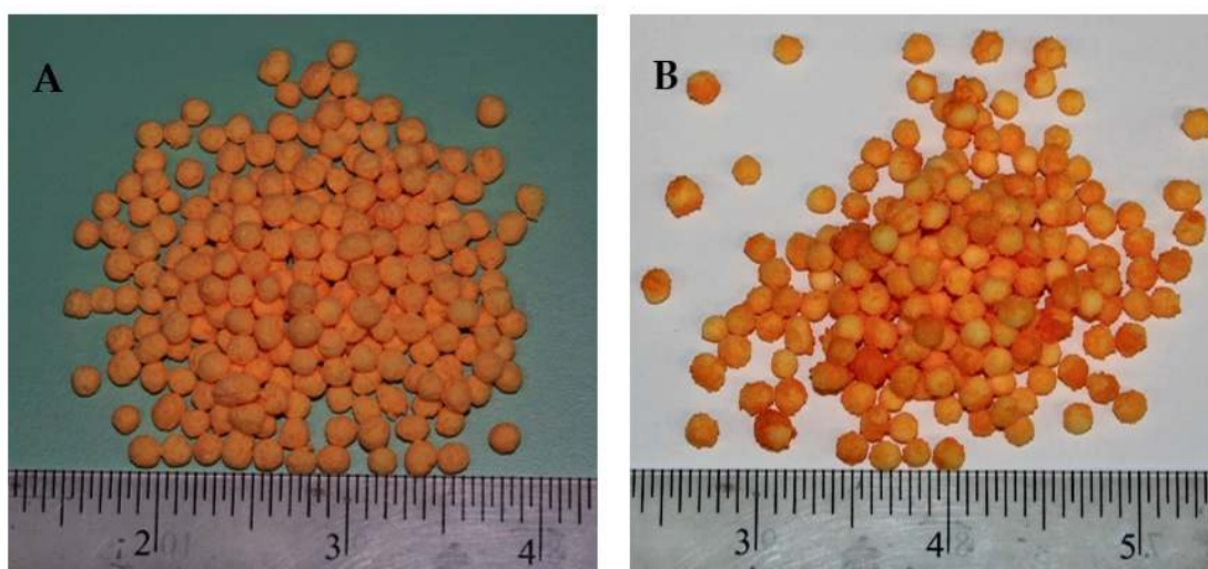
Figure 8. SCU samples achieved at (A) moderate T_{\text{fluid}} and P_{\text{atom}} and (B) higher T_{\text{fluid}} and P_{\text{atom}} .
