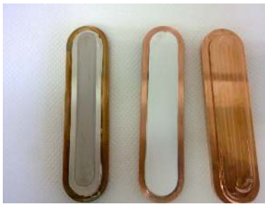
Figure 2. Target support: On the right, without electroplating; In the middle, silver electroplated; On the left, nickel electroplated on silver layer.
