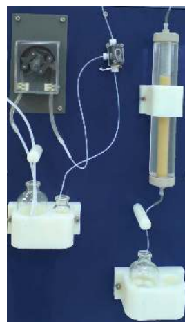
Figure 7. Separation and purification unit.
