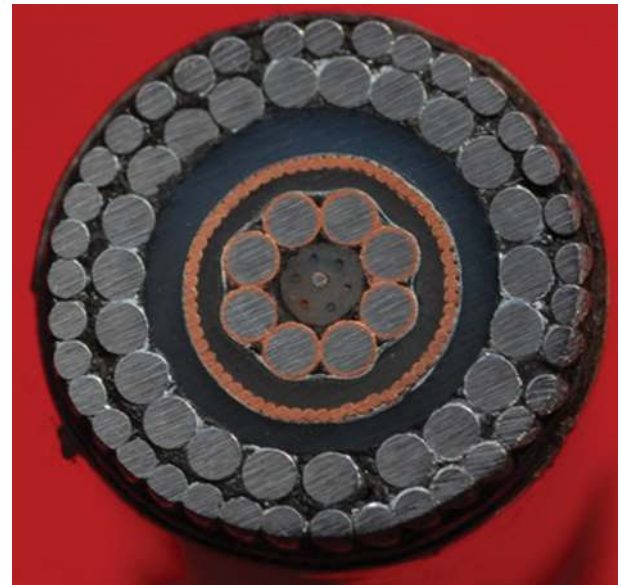
Fig. 6. Cross section of the DISC drill's fiber-optic cable.
