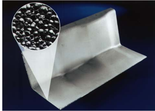
Fig. 10: 3d-shaped sandwich of an aluminium foam with aluminium face sheets (width 1000mm, thickness 8 mm)
