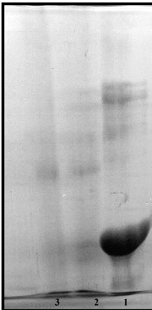
Figure 1. SDS-poliacrilamide gel electrophoresis pectin lyase from Bacillus pumilus ; (1) standart proteins, (2) purified pectin lyase by DEAE cellulose ion exchange chromatography, (1) purified pectin lyase by gel filtration chromatography.
