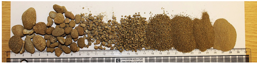
Figure 5. Visual representation of the particle size distribution of the produced clinker. The scale divisions on the rule are in centimetres
