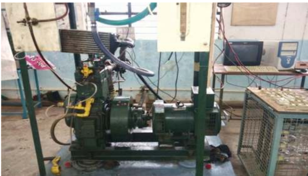
Figure 1. Four stroke Single Cylinder CI engine with electrical loading.
