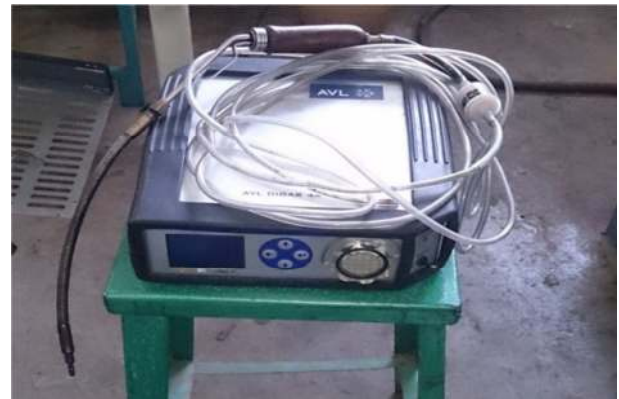
Figure 2. Exhaust gas analyser.
