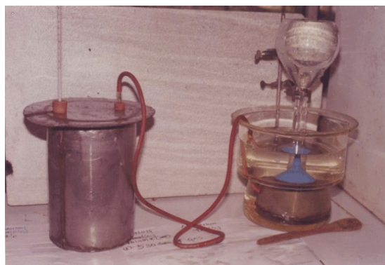
Fig. 1: A 10-L laboratory type anaerobic digester used for the investigation
