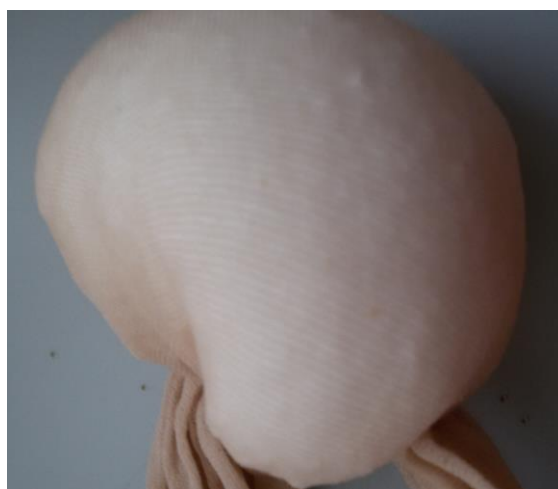
Figure 15 - Image of the second particles set up.: PP-PEI/PSS/BDMDAC-1-hour-of-contact particles inside the tissue netting (“net-trapped particles”).
