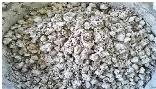
Fig. 8. Concrete sample mix with 16% rubber crumb
