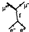
Fig. 5. Production of a single excited muon through one-photon intermediate state in an e^-e^+ collision.
