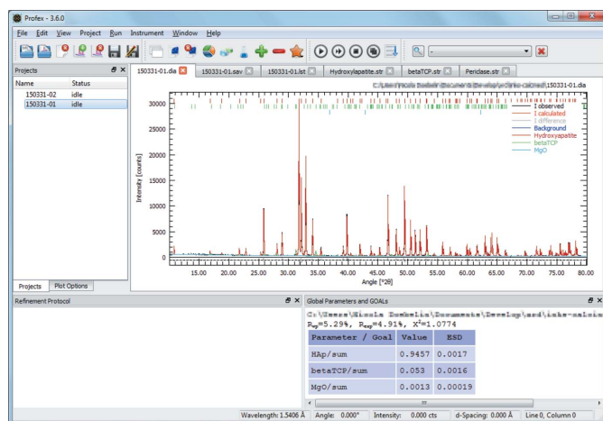
Figure 1 The Profex main window, showing the central plot display area with tabs of open text editors at the top, as well as several lists and output consoles docked and stacked left and below the plot display area.
