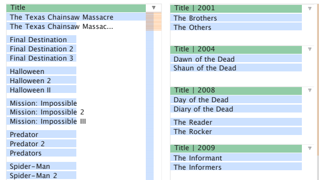
Figure 4: Conditioned duplicate detection. Left: Movie titles clustered by Levenshtein distance reveal over 200 potential duplicates. Right: Conditioning the clustering routine on ‘Release Year’ reduces the number of potential duplicates to 10.
