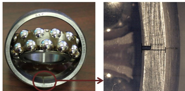
Figure 3-6 SKF 1205 ETN9 with a seeded fault
