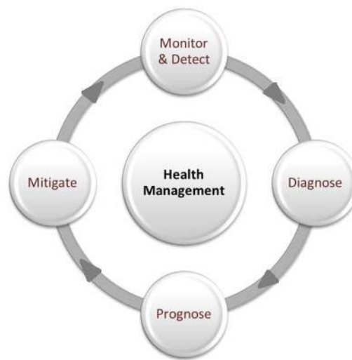
Figure 1-1 A typical PHM system
