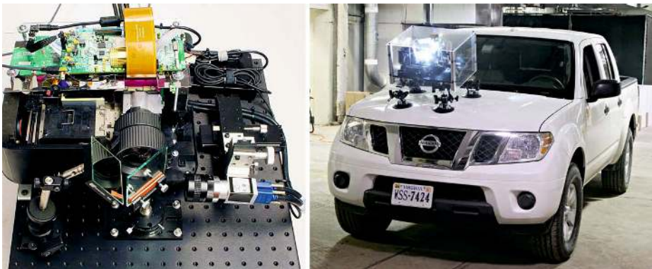
Fig. 1. Left: Prototype of our programmable automotive headlight design (computer not pictured). The camera, spatial light modulator, and beam splitter are firmly mounted to an optical breadboard. A mirror to the side of the beam splitter deflects reflected light from the light source upward. Right: Road tests were conducted by securing the prototype to the hood of a vehicle with a suction cup-based mount. An acrylic enclosure was constructed to protect components from dust, dirt, and moisture.
