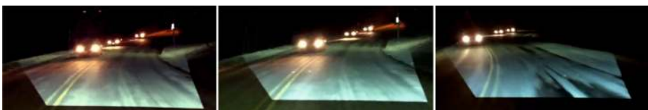
Fig. 6. View shown from the perspective of the vehicle equipped with our prototype. Left: Anti-glare feature is disabled acting as a typical high beam. Middle and Right: Anti-glare feature is enabled detecting multiple oncoming vehicles and reducing light only in the direction of each driver. Notice no discernable difference between images.
