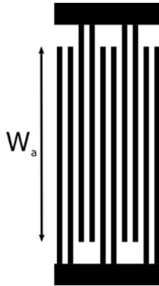
Figure 3.9: Illustration showing the beamwidth for a transducer as defined by the overlap between positive and negative electrodes. A double-electrode transducer is shown but this definition is the same for all electrode patterns discussed in this dissertation.
