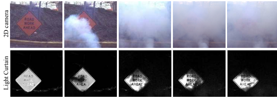
Fig. 7. Seeing through volumetric scattering media. Light curtains suppress backscattered light and provide images with improved contrast.
