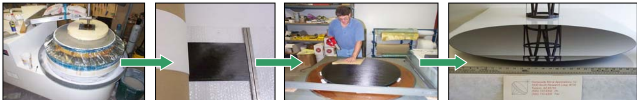
Figure 1. CFRP fabrication sequence from left to right, processing the glass mandrel, CFRP prepreg material, lay-up of prepreg over the glass mandrel, processing and release CFRP mirror from the mandrel, ready for coating.
