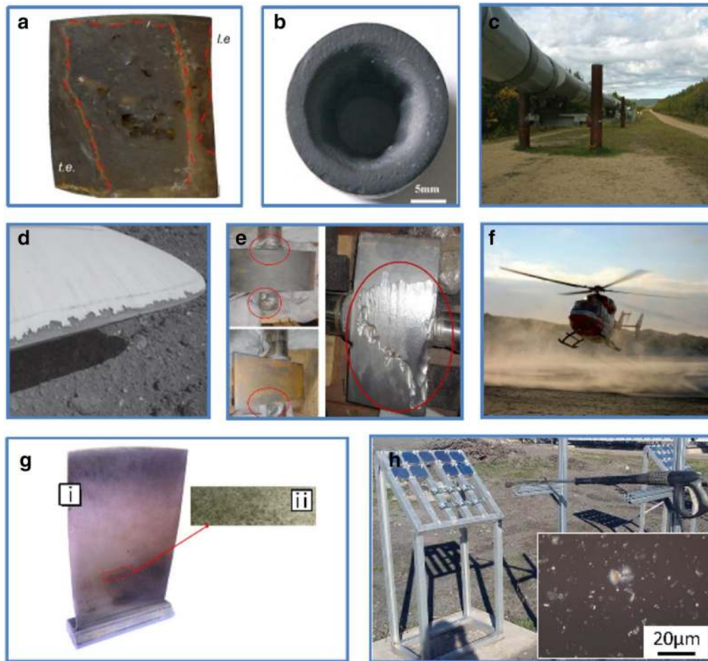
Figure 17 (a) The erosion phenomenon of a fan blade [7]; (b) The erosion behavior of a ceramic nozzle [138]; (c) Conveying pipelines of oil or gas; (d) The erosion phenomenon of a wind turbine blade [144]; (e) Sediment erosion of hydroelectric generator blades [143]; (f) Sand impact on working helicopter blades; (g) The erosion phenomenon of a compressor blade: (i) A blade of compressor [149], (ii) Pits caused by solid particle erosion in the critical zone [149]; (h) The cleaning setup of antireflective glass coatings eroded by a sandstorm; microscope picture of a sample with antireflective coatings after treatment in the sandstorm chamber (inset) [157]
