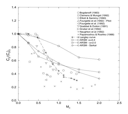
FIG. 8. Effect of compressibility on normalized thickness growth rate, ARSM calculations of a mixing layer.
