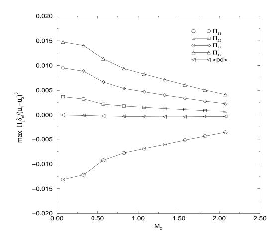
FIG. 6. Variation with convective Mach number for the mixing layer; the pressure-strain tensor. [ $\alpha = 1.2$ ]
