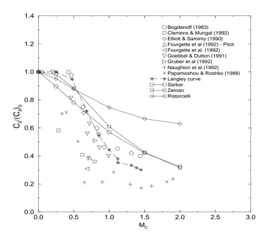
FIG. 7. Effect of compressibility on normalized thickness growth rate,  $k - \epsilon$  calculations of a mixing layer.[ $\alpha = 2$ ]
