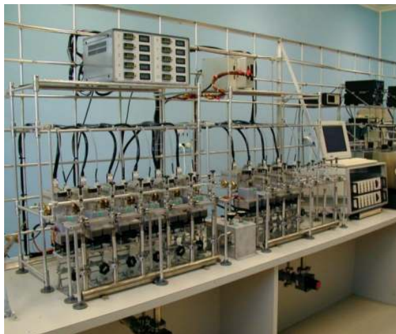
Figure 3a The new graphitization system dedicated to small samples
