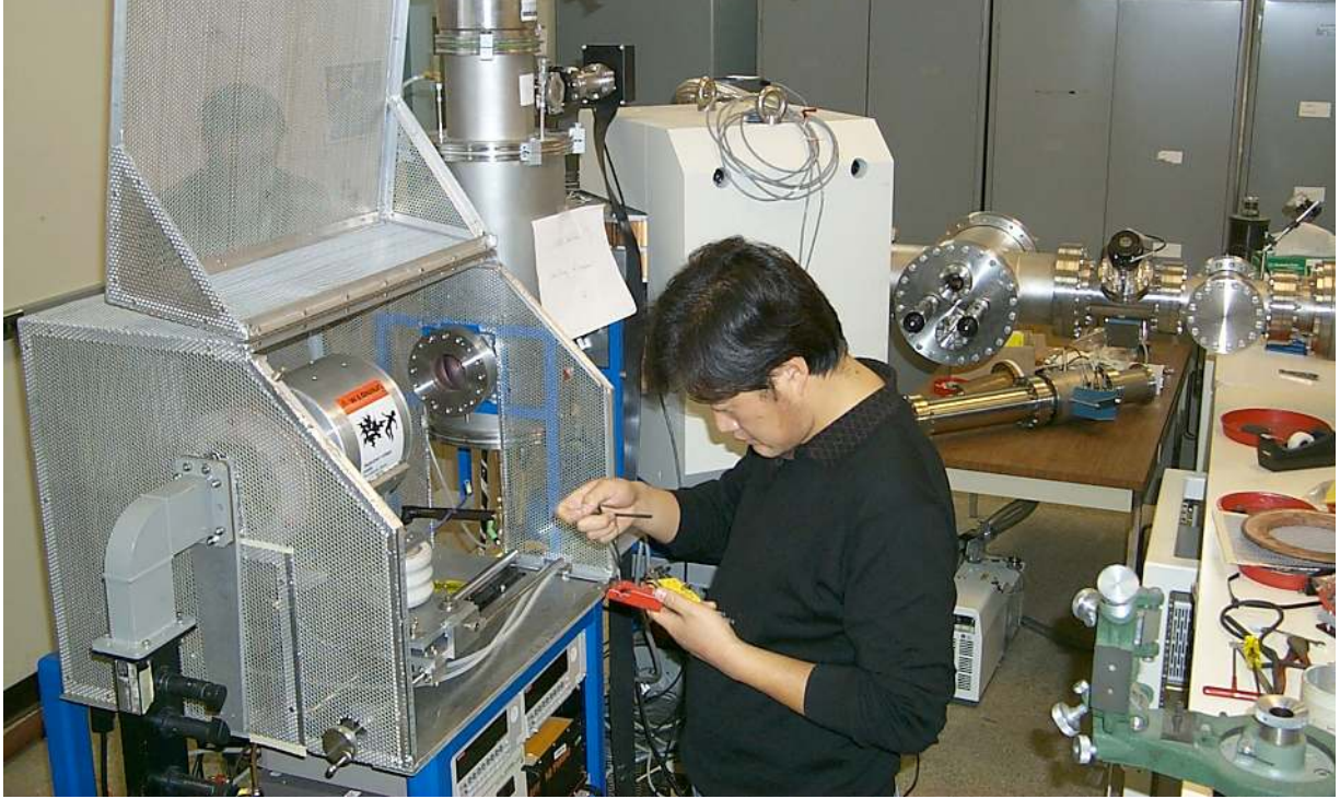
Figure 2. The ion source mounted on the ion-source test stand. The ion source is to the left inside the cage and the double focusing magnet is back center.
