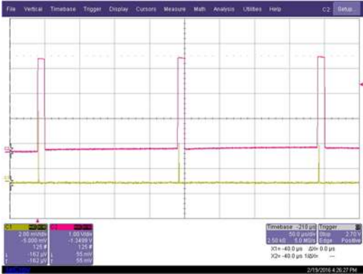
Figure 2. An oscilloscope record of the temporal profile of the triple-pulse generation (yellow) as compared to the Q-switch timing signal (red).
