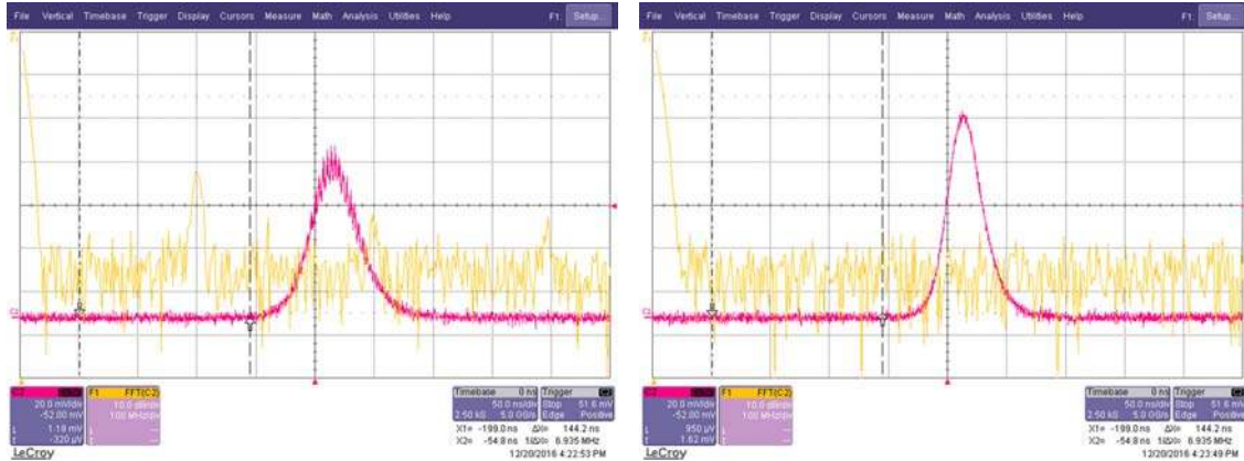
Figure 7. An oscilloscope records comparing the temporal profiles (red) and frequency spectrum (yellow) of the un-seeded (left) and seeded (right) pulsed laser output. These records were obtained for the first pulse.
