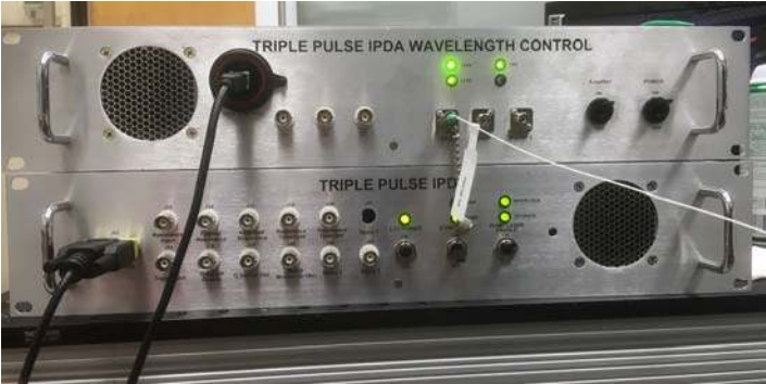
Figure 1. Frontal picture of the triple-pulse IPDA Laser Timing Control (LTC) unit (bottom) and Wavelength Control Unit (WCU) (top) packaged end-products. Both units are rack mountable, flight hardened, and were tested successfully.
