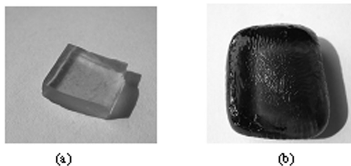
Fig. 14 TSGE based on PAA-PEG system before (a) and after (b) soaking in liquid electrolyte.
