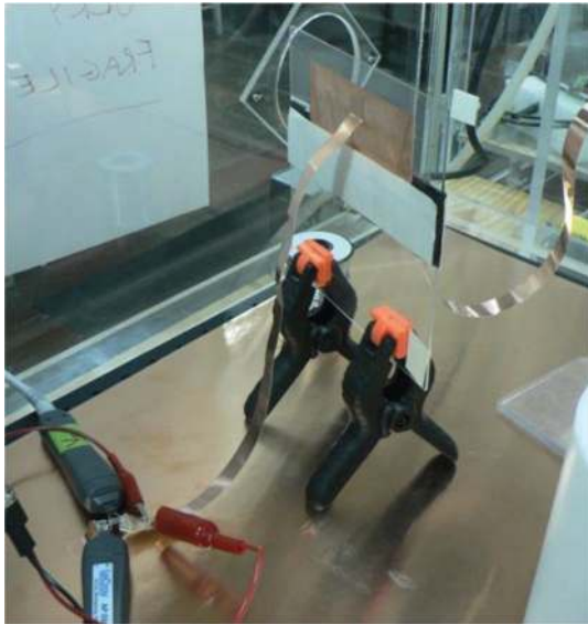
Fig. 7 Experimental setup, showing actuator test article viewed from the covered electrode side, copper ground plane, flat copper tape leads, and capacitor-resistor assembly with differential probes attached.
