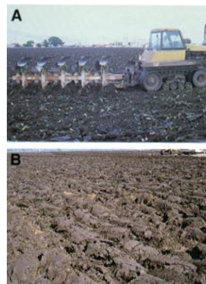
Fig. 9. (A) A Wilcox plow adapted for deep plowing. (B) Large clods formed as a result of deep plowing in a commercial field.
