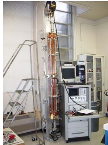
Figure 11: Wire measurement set-up with the RDDS1 structure.
