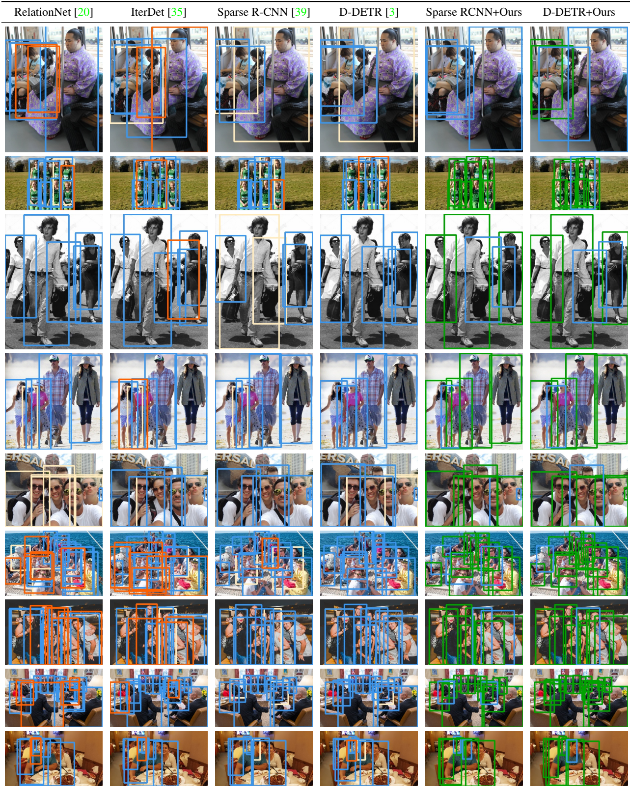
Figure 9: Results visualization of RelationNet [20], IterDet [35], Sparse RCNN [39], deformable DETR [54] and our approach based on them [39, 54]. Blue boxes are true positive detections, light yellow boxes are missed instances and orange boxes are false positives. Green boxes represent progressively refined detections in our method.
