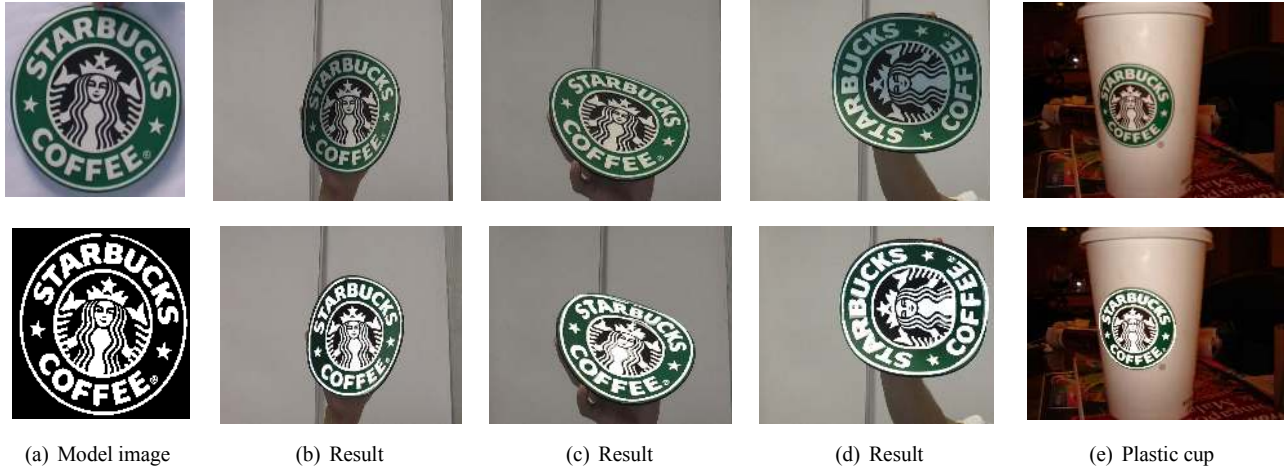
Figure 3. We use a Starbucks pad as the deformable object. The model image is shown in (a) the contour of the model image is extracted using a simple gradient and filling operator, which is overlaid on the input image. (b) to (d) show the results. (e) shows the result where the pad is replaced by a plastic cup. The model contains 120 vertices, and the whole process, including image capturing and rendering, runs around 18 frames per second. More results are included in the supplementary material.
