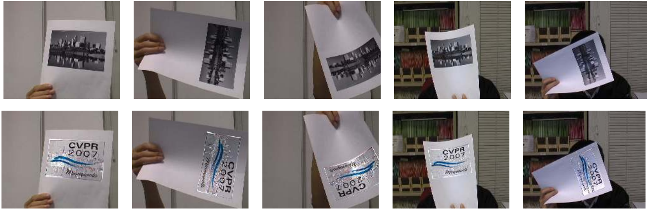
Figure 6. Re-texturing a picture on a piece of paper. The first row is the 720 \times 576 images captured by a DV camera. The second row is the results of replacing the picture with the CVPR logo.
