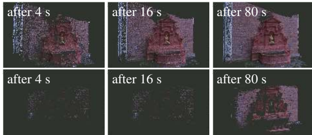
Figure 7: One to one comparison of the patch growing between the proposed method (top) and PMVS (bottom).
