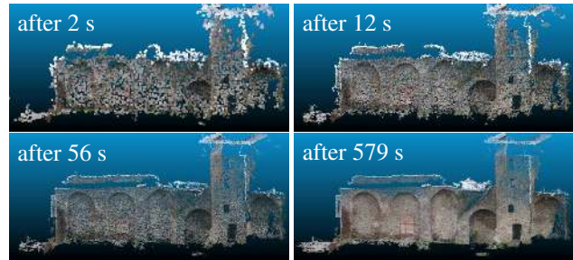
Figure 1: Progressive reconstruction of the citywall dataset (562 images). With increasing runtime, the resulting dense point cloud gets more accurate and covers finer details.
