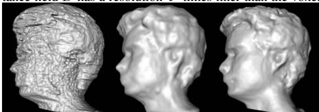
(a) space carving (b) level set (c) our method Figure 5. Comparison. Space Carving [21] fails to build a satisfying approximation (a) (to achieve a fair comparison without aliasing, the voxel volume has been triangulated using the Marching Cubes [25]). The level-set technique [23] builds a less detailed geometry (b) compared to ours (c); e.g. observe the chin, eyes and forehead.
