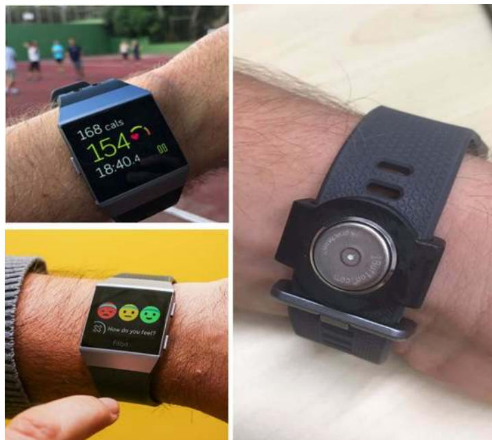
Figure 2. Fitbit Ionic and sensor attachments deployed here for monitoring of (a) temperature and humidity of air in the proximity of human body, (b) heart rate, skin temperature, and humidity at wrist, and (c) activity level and momentary feedback. Two iButton sensors [38] are placed on the watch strap using a 3D printed harness. The Fitbit activity trackers used have a 3-axis accelerometer to track the wearer's motion patterns (e.g. those that indicate walking, swimming or cycling) to approximate the number of steps taken, calories burned, floor climbed, and length of time performing exercises. The PurePulse (photoplethysmography) technology for heart rate monitoring [36, 37] uses LED lights installed at the back of the instrument to detect blood volume changes that are due to capillary expansion and contractions, and has been shown to tracks heart rate well when compared to three-lead electrocardiography [37]. The design and use of the smartwatch app will be further discussed in future studies.
