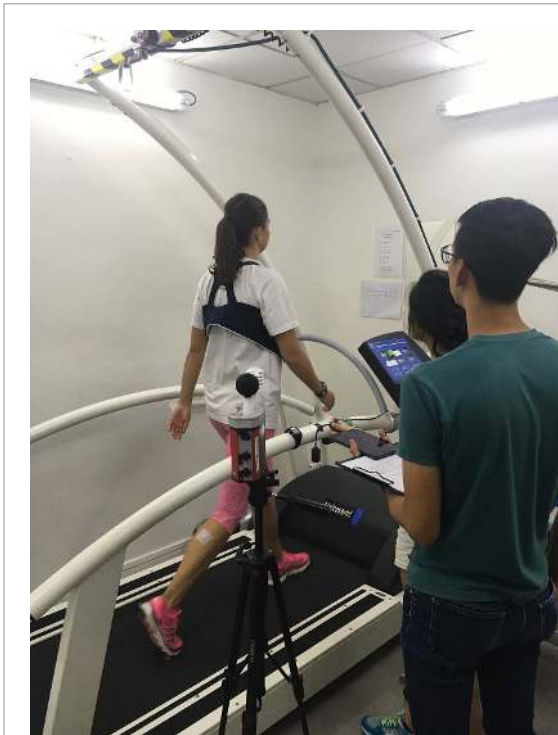
Figure 3. Controlled-environment experiment at NUS Department of Physiology. A participant is walking on a treadmill while wearing the wrist-mounted sensor arrangement (figure 2), chest-wrapped heart rate monitoring (Polar A300), and iButton sensors for recording skin temperature at various body parts. The environmental parameters in the climate chamber as well as ratings of thermal sensation (ASHRAE's 7-point scale) and RPE are continuously monitored throughout the experiment. Data from the ingested telemetric capsules were collected by the wireless data-recording devices and the body core temperature is monitored closely such that the experiment is ceased if the threshold of 40 °C is reached.
