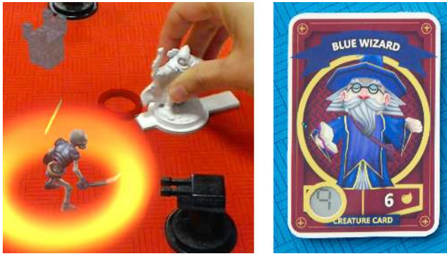
Figure 7. The Tower Defence game combines tangible input with augmented reality holograms (left). Segmented E-Ink displays embedded in playing cards are driven by a power-harvesting I/O Tag (right).
