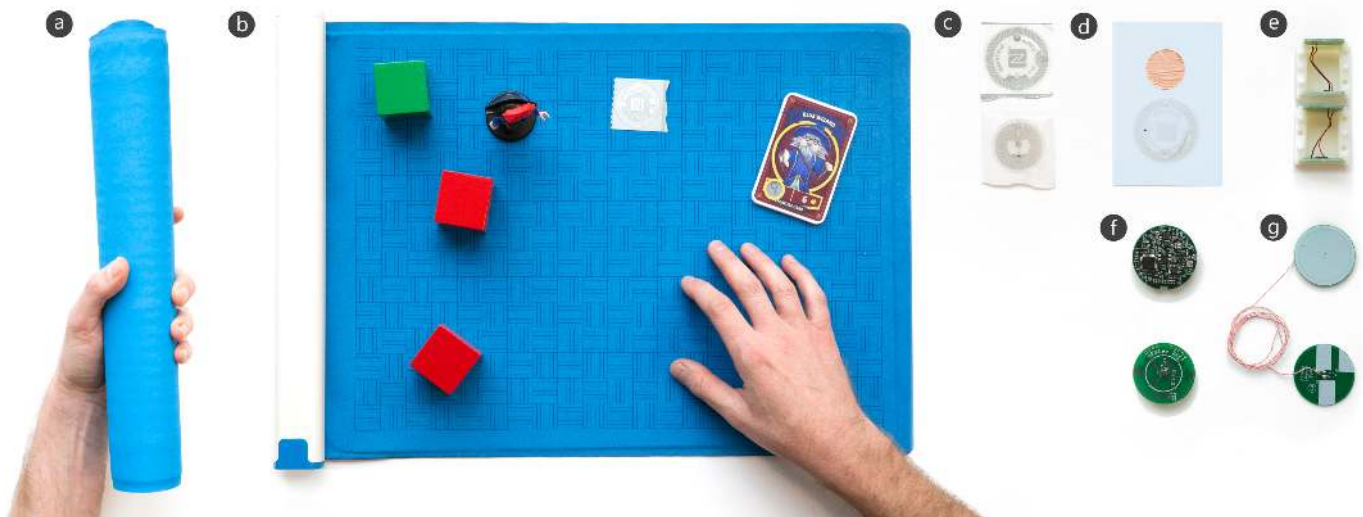
Figure 1. The Zanzibar Mat (b) tracks objects equipped with NFC tags (c), senses touch, detects hover gestures, and can be rolled up for portability (a). Different tag designs can be used to determine rotation (d), stack objects (e), provide I/O (f), and extend sensing outside the bounds of the Mat (g).
