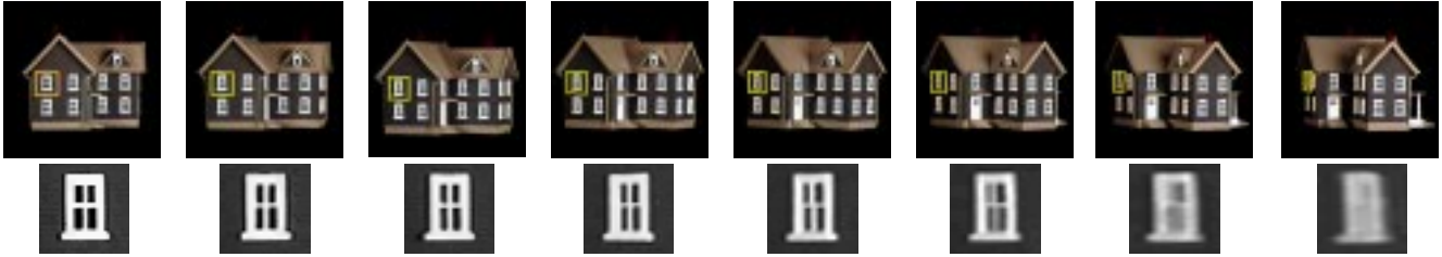
Figure 2: Projective tracking in a QuicktimeVR object movie (a sequence of still images). The bottom row shows the warped region ( I_1' ).
