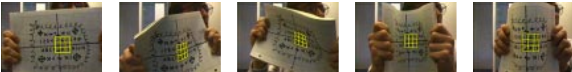
Figure 4: Frames from tracking a flexing object using a 48x48 piecewise projective patch with a 3x3 grid.
