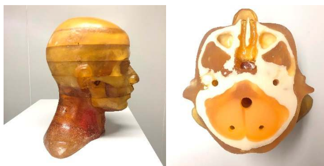
Figure 4. Real data experimental phantom: Chengdu Dosimetric Phantom, CPET Co. Ltd., Chengdu, China.
