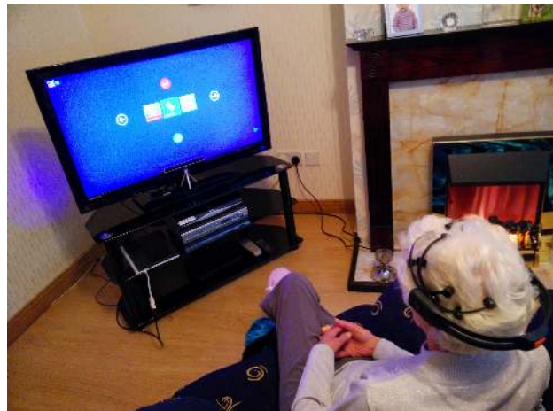
Fig. 2. A representative subject using the implemented system in order to complete the three tasks within a smart home using the Emotiv EPOC and the EyeTribe tracker together
