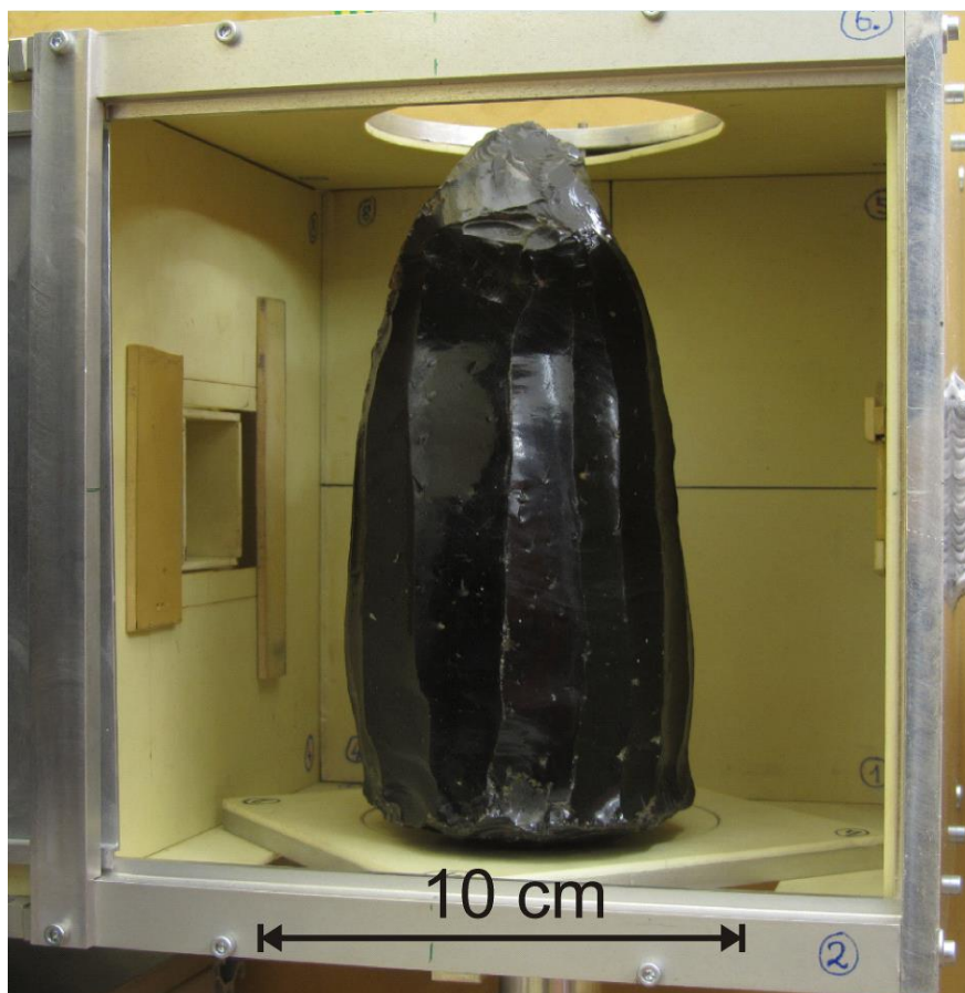
Figure 4. An obsidian core in the sample holder of the Budapest NIPS-NORMA station.
