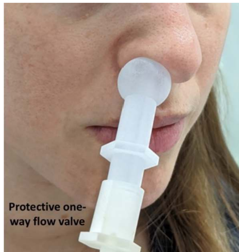
Fig 2. A one-way disposable sampling valve protected participants. The sampling valve fits snugly against the nostril, providing an air-tight connection for pulling air from within the nostril, independent of exhalation. The person in the image is a co-author demonstrating, and not a participant, and informed consent for publication of identifying images in an online open-access journal was obtained.
