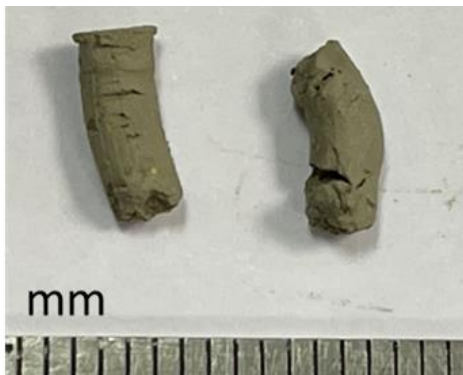
Figure 1. 3 mm diameter cylindrical shape ‘green’ granules.
