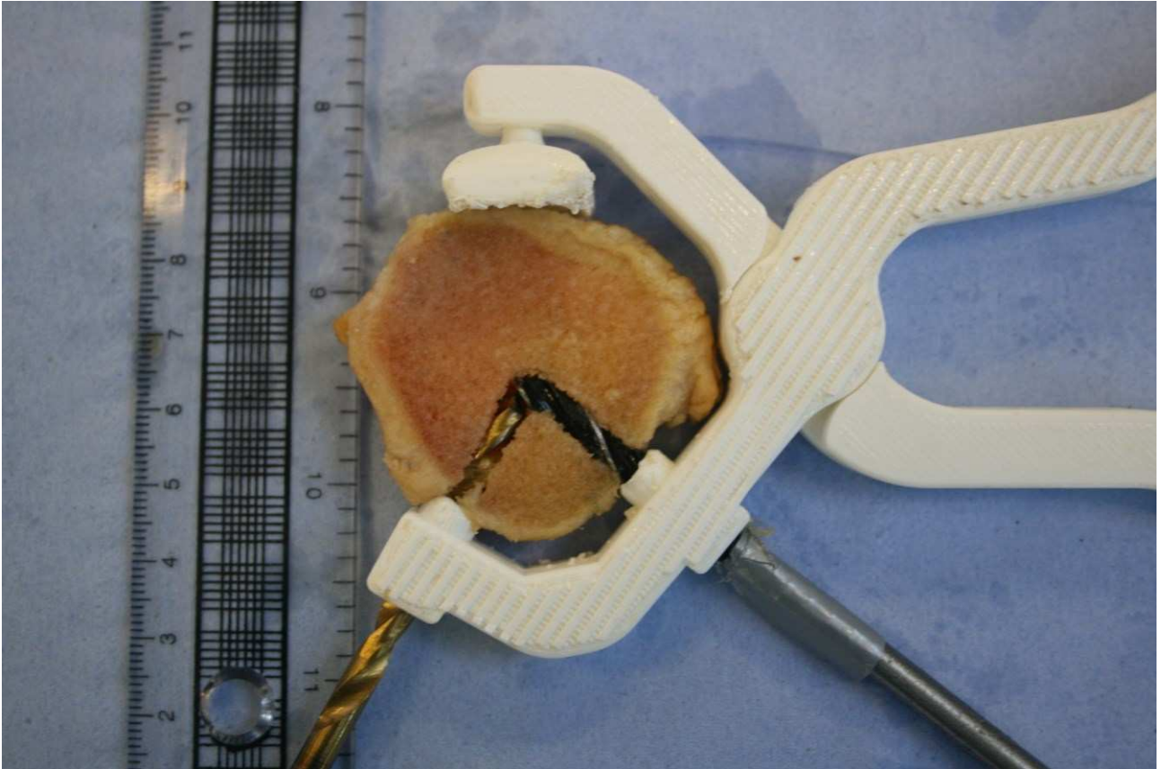
Figure 5: Image showing a cadaveric patella divided in the coronal plane with the MPFL drill guide and two drill bits in situ for illustration purposes. Note that owing to limitation in 3D printer size we only had a small drill guide available, when for this particular patella a larger size would have been more appropriate.
