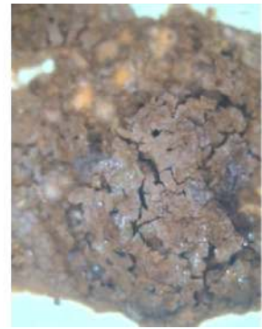
(c) The same rust after drying
