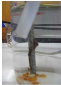
(a) Initial ocalized corrosion showing that the rust is falling down and is gelous
