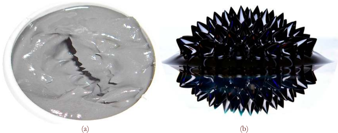
Figure 2: Magneto rheological fluid (a) from Lord [1] and ferrofluid (b), produced by [2].
