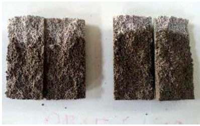
Fig. 6. Mixture 2 specimens after capillary water absorption test.
