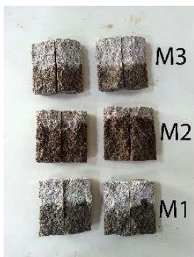
Fig. 9. Capillary rise of the mixtures 1, 2 and 3.
