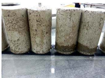
Fig. 2. Water absorption by capillarity test.
