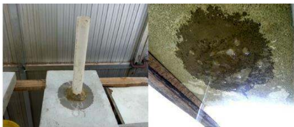
Fig. 13. Water permeability test of the plates with the Mixture 6.
