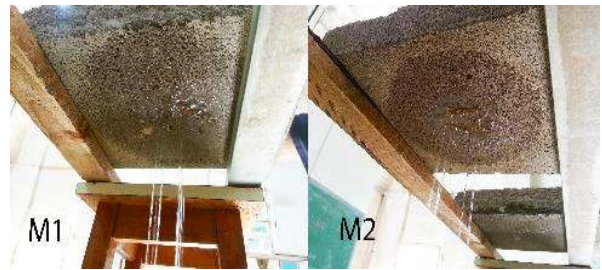
Fig. 10. Permeability test for Mixtures 1 and 2.
