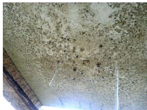
Fig. 12. Water permeability test of the plates with the Mixture 5.
