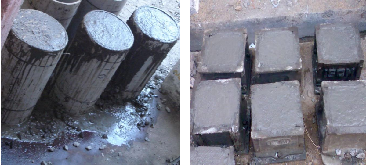
Figure 1. Casting of Specimen
