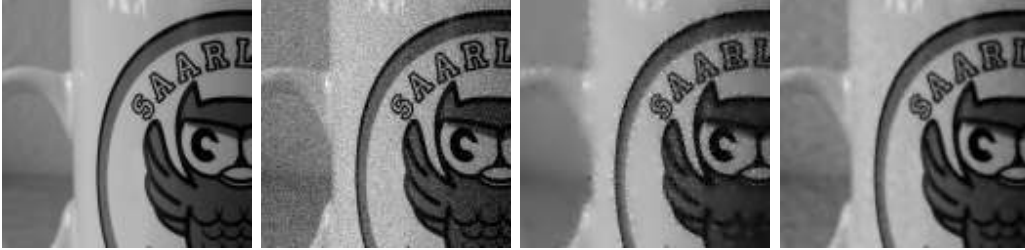
Figure 2: Higher order nonlinear diffusion with g(s^2) = 1/(1 + s^2/\lambda^2) . Top left: Original image, 256 \times 256 pixels. Top right: With additive Gaussian noise, standard deviation \sigma = 10 . Bottom left: Method by You and Kaveh [55] without postprocessing, \lambda = 2.5 , t = 100 . Bottom right: Method by Lysaker et al. [27] \lambda = 0.01 , t = 6 .
